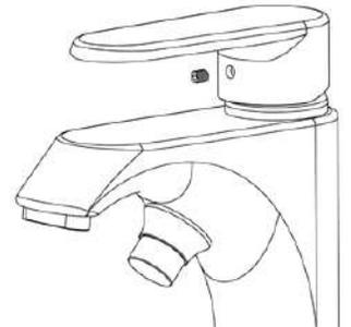
Step.3 Take out the handle and remove the brass escutcheon
