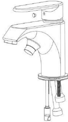
Step.2 Use an Allen wrench to remove the handle Screw.
