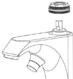
Step.4 Use a wrench to unscrew the pressure cap.
