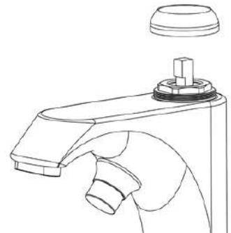
Step.5 Remove the cartridge and replace it with new piece.
